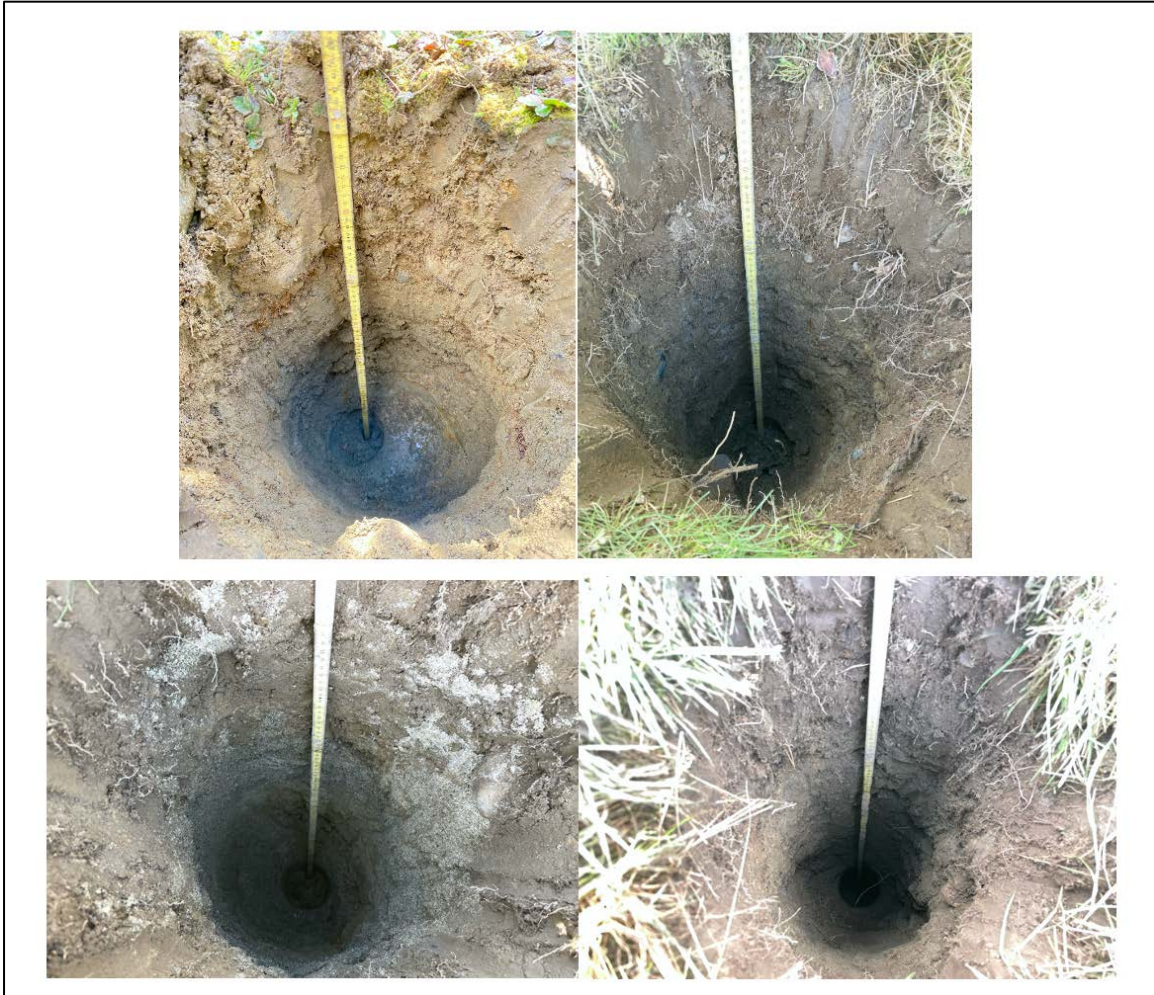
Figure 23. Subsurface deposits identified at the project location. Clockwise from upper left, images are of intact soil horizons overlying glacial till (probes #1) and disturbed soil horizons overlying glacial till (probe #2, 3, and 4).
